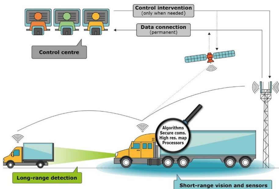
Figure 7: Stylised driverless truck operating environment with optional Control Centre (ITF 2017).
